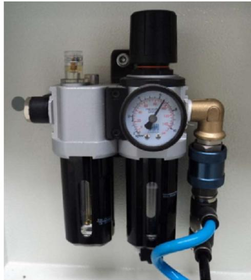
Picture 6.4: Air Lubricator Unit
