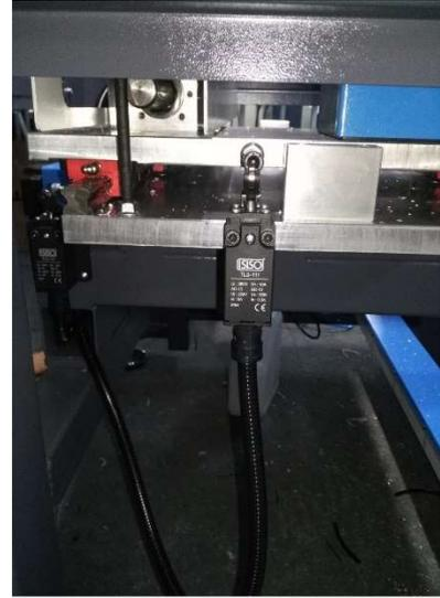
There are mechanical switches at the reference points of the 3 axes of the machine. When any situation is encountered, when the machine is sent to the reference from the screen, the machine will go to its original position, that is, to the zero point. If the axis passes the mechanical switch when it is moved by manual control. Mechanical Stoppers, whose zero point is out of bounds, will stop the axis.
