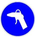
This symbol indicates that an air gun must be connected to the air outlet where it is used
