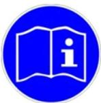
This symbol indicates that the machine should not be operated before reading the operating manual and fulfilling the necessary conditions.
