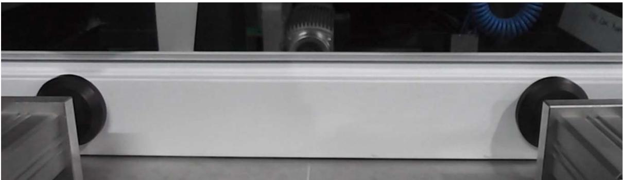
There are 2 clamping pistons on the machine to perform operations on aluminum and PVC profiles. The machine will not start unless the profile is fixed.
