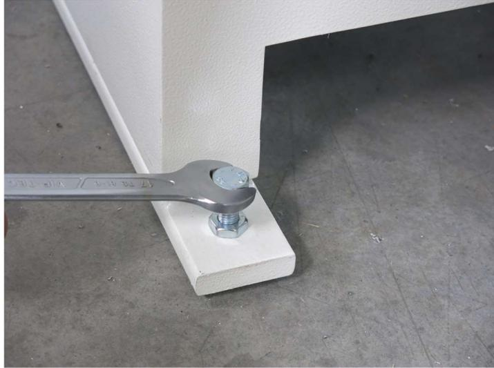
Figure 6.5: Balancing the Machine with the Help of Setting Bolts
