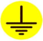
This symbol indicates that the connection it is used for is the ground line.
