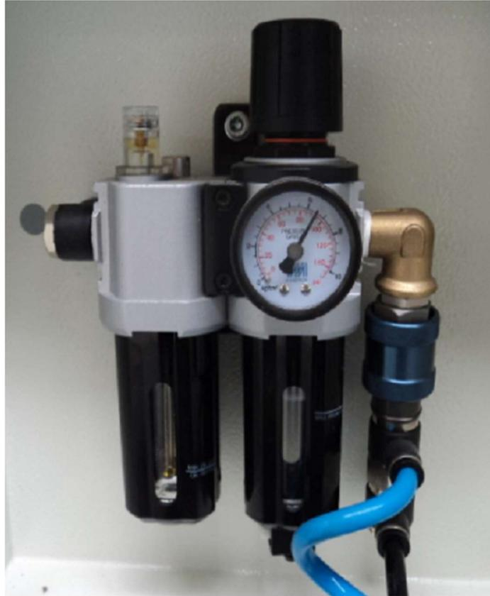
Picture 8.2: Air Lubricator (Lubrication)
