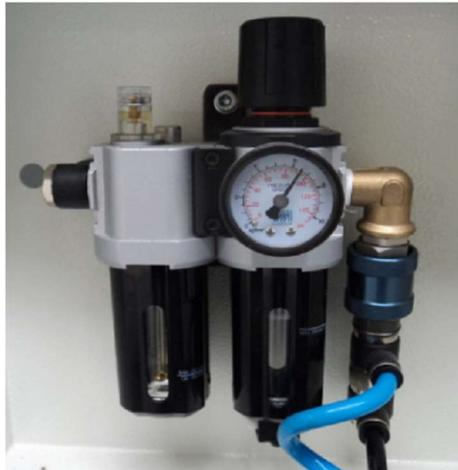
Picture 7.1: Air Lubrication Unit
